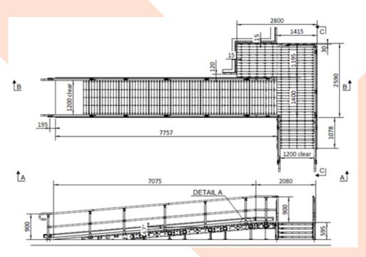
We would recommend specifying the Ezibilt ramp in 600mm increments, as the system is put together with a combination of modules to suit the site requirements.
